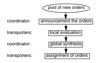
Figure 5: Phases of the Scheduling Algorithm
