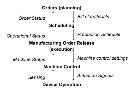
Figure 7 Typical Manufacturing Control Hierarchy
